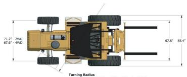
Turning Radius 2WD with brakes 10'-7" 4WD with brakes 10'-7" 2WD without brakes 12'-5" 4WD without brakes 12'-9"
